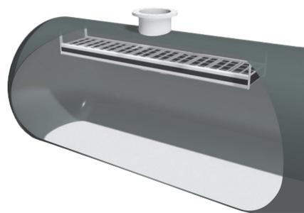
*In a typical steam drum, mist eliminators properly located below the outlet nozzles assure high steam purity.*
