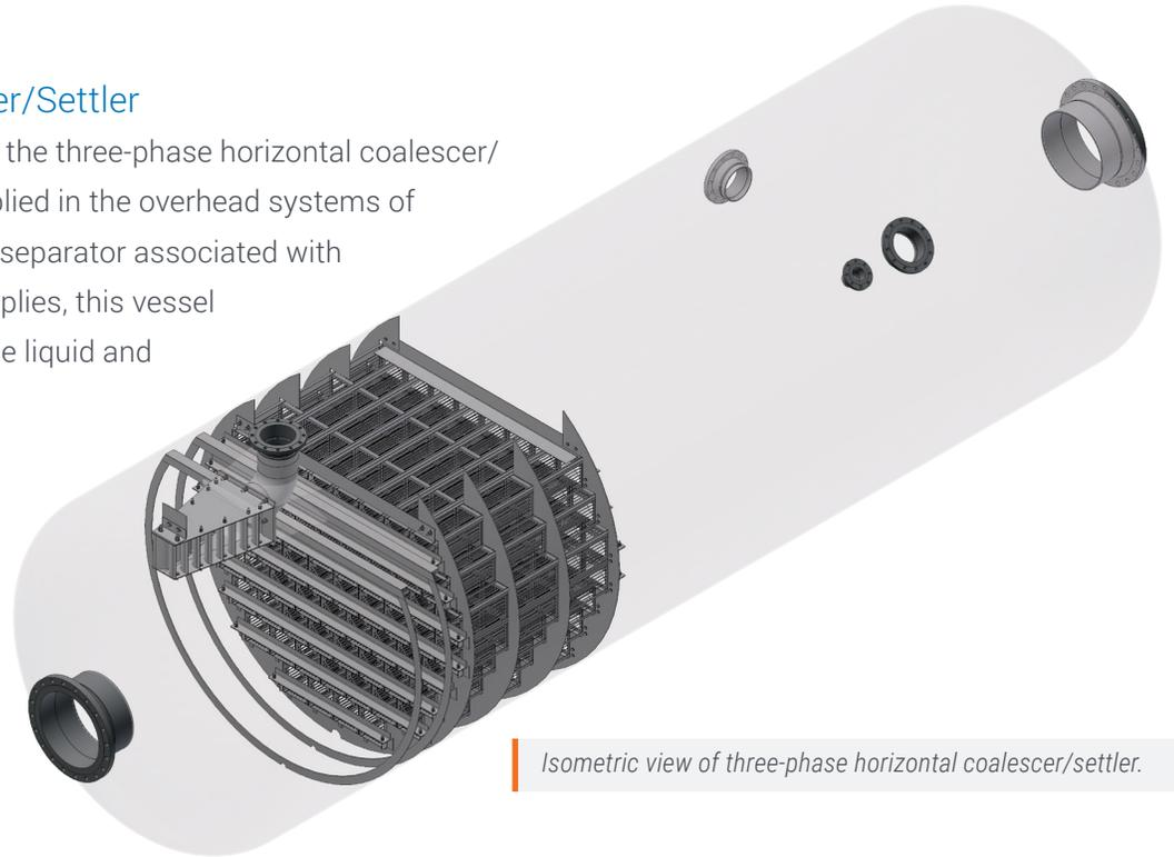
*Isometric view of three-phase horizontal coalescer/settler.*
