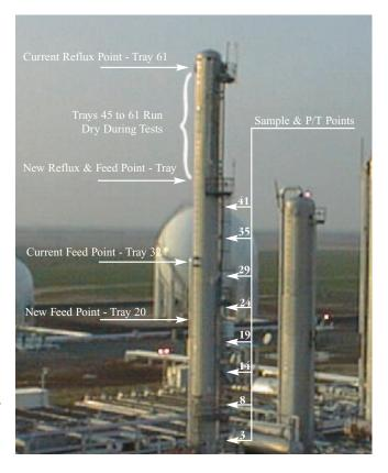
for ULTRA-FRAC trays. With this *Test and Demonstration* unit, we can confidently predict ULTRA-FRAC efficiencies.
