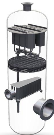
Vertical-flow DEMISTER-PLUS type MC-V separators use VORSOMAX mist eliminators for higher capacity. Solutions also available for horizontal separators.
