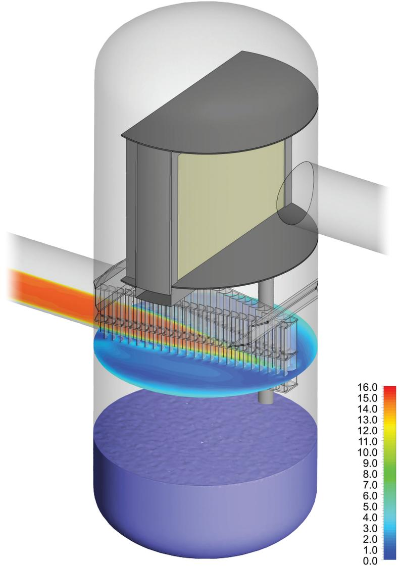
The case illustrated below was a study of the velocity patterns inside a critical separator vessel operating under vacuum. For optimal performance, it was important that the velocity profile through the mist eliminator be uniform. The CFD study confirmed this to be the case, based on the vessel geometry.
