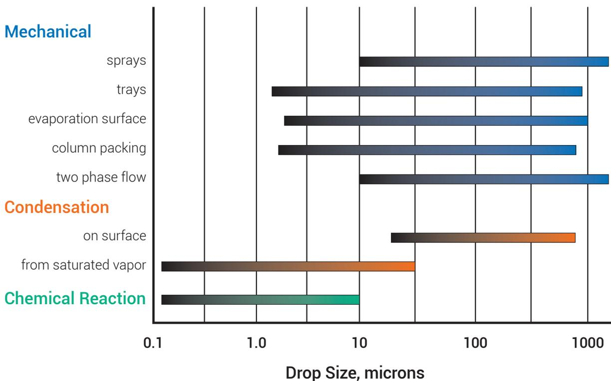
**Mechanical:** Experience shows that droplets generated by mechanical means are commonly 5-10 $\mu$  and larger in diameter. But a boiling or bubbling liquid surface will form droplets down to just a few microns in diameter.
