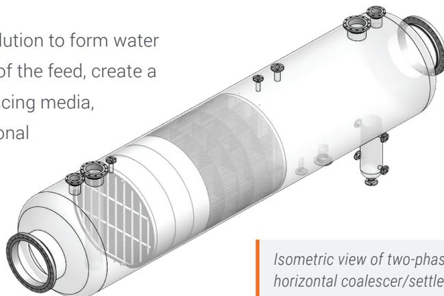
*Isometric view of two-phase horizontal coalescer/settler.*
