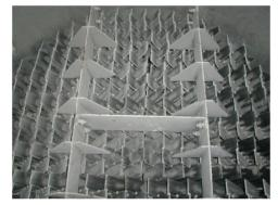
KFBE catalyst stripper packing after 3 years operation
