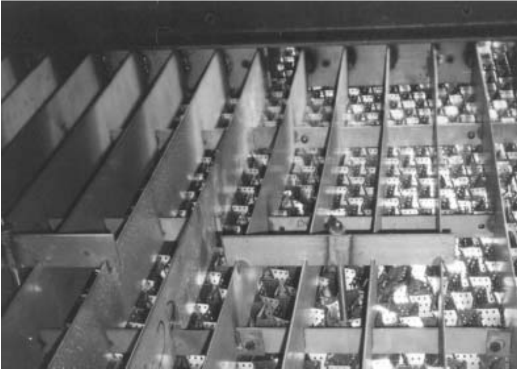
Figure 9: Packed Bed Hold Down Using Through Rods
