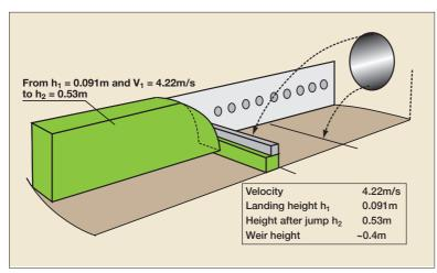
Figure 3 Hydraulic jump calculations for existing liquid inlet
