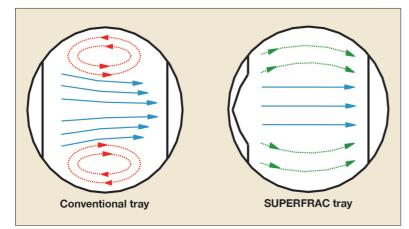
**Figure 7** Liquid flow distribution comparison between conventional trays and multi-chordal Superfrac tray
