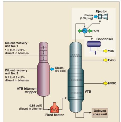
Figure 1 Simplified process flow diagram (the pink tower is the steam stripping tower)
