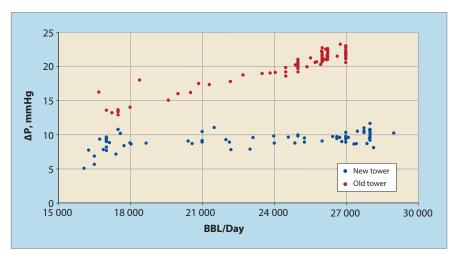
Figure 5 Column pressure drop vs feed rate, all feedstocks
