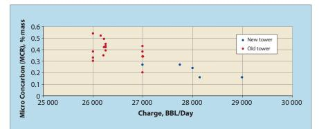
Figure 7 Micro Concarbon (MCR) in HVGO comparison for API 16-17 feedstock
