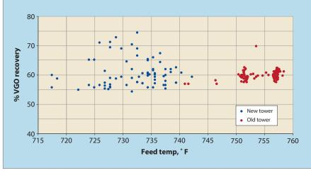
Figure 6 Gas oil recovery comparison for API 16-17 feedstock
