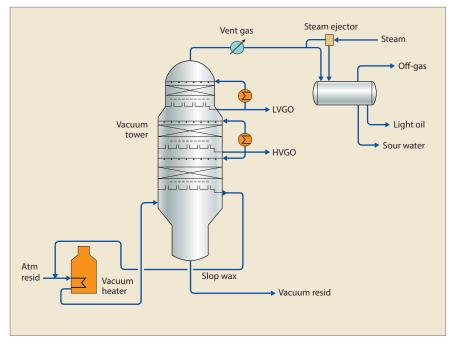
Figure 1 Schematic of a typical dry vacuum crude unit
