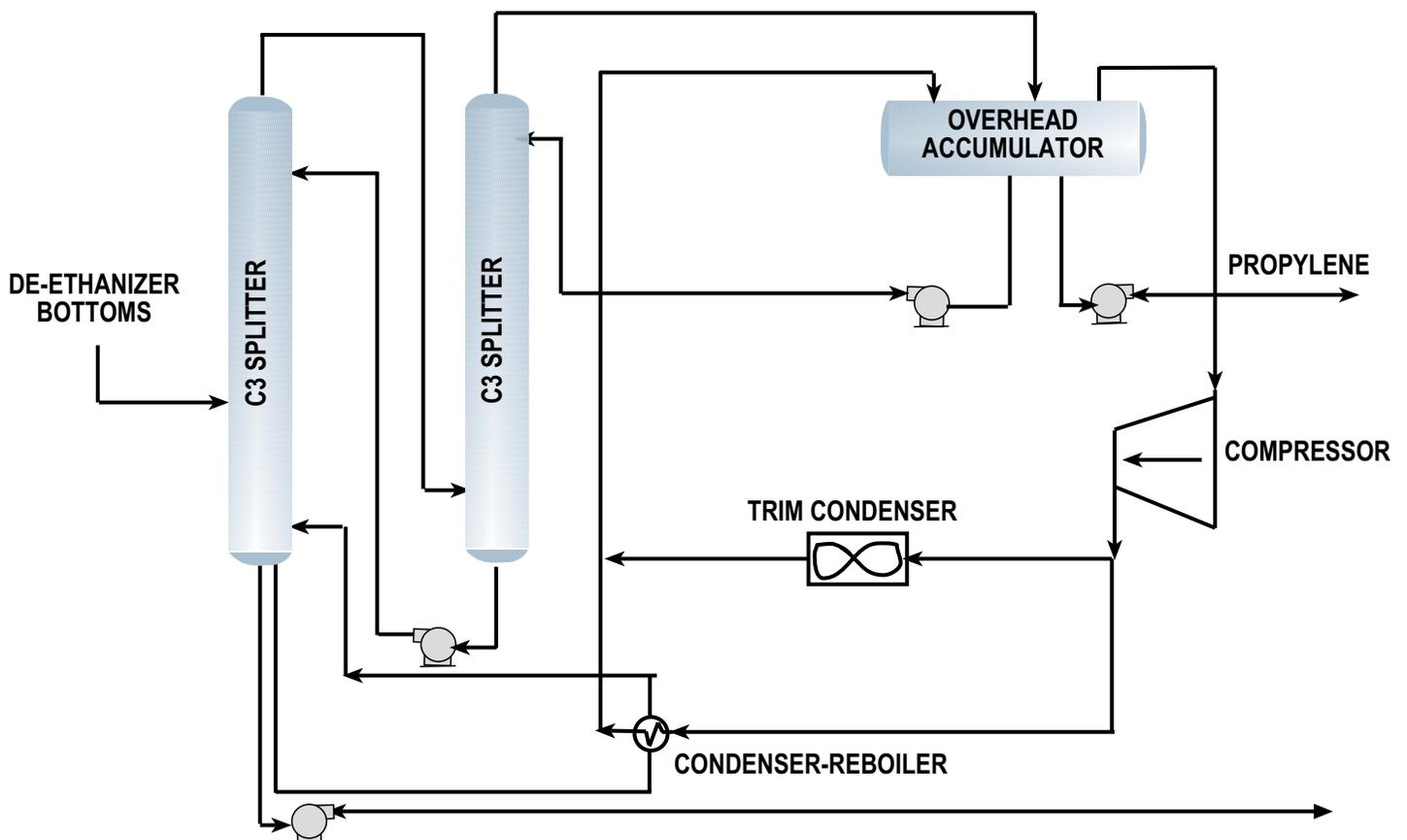
C<sub>3</sub> Splitter Simplified Process Flow Diagram
