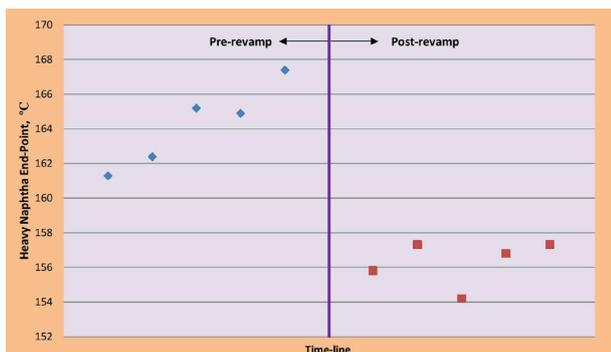
**Figure 6.** Combined HCU/DHT stripper heavy naphtha endpoint.
