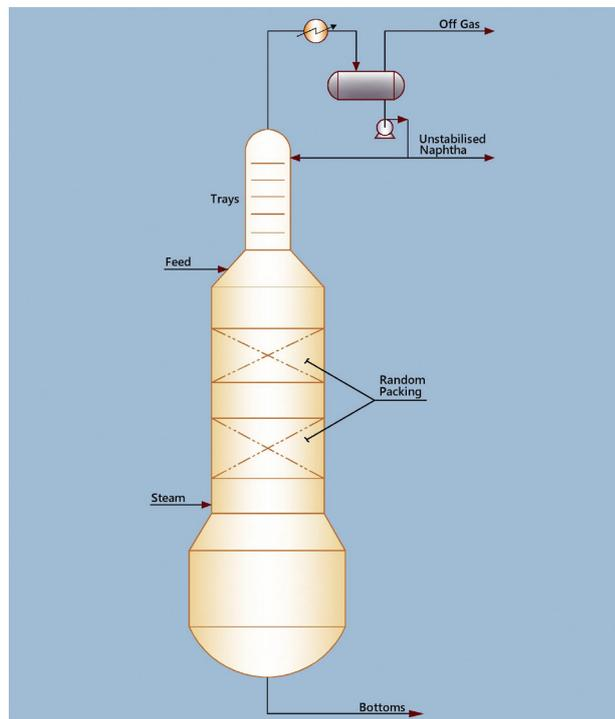
**Figure 1.** A hydrocracker/DHT stripper.
