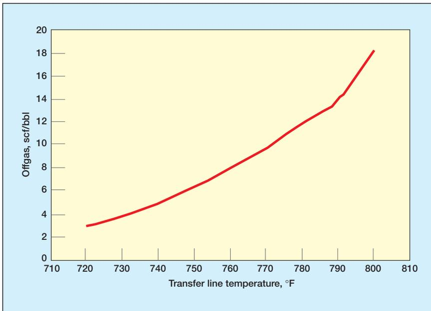
**Figure 2** Graphical representation of Lieberman relationship; measured plant variables, transfer line temperature and off-gas-to-crude flow ratio
