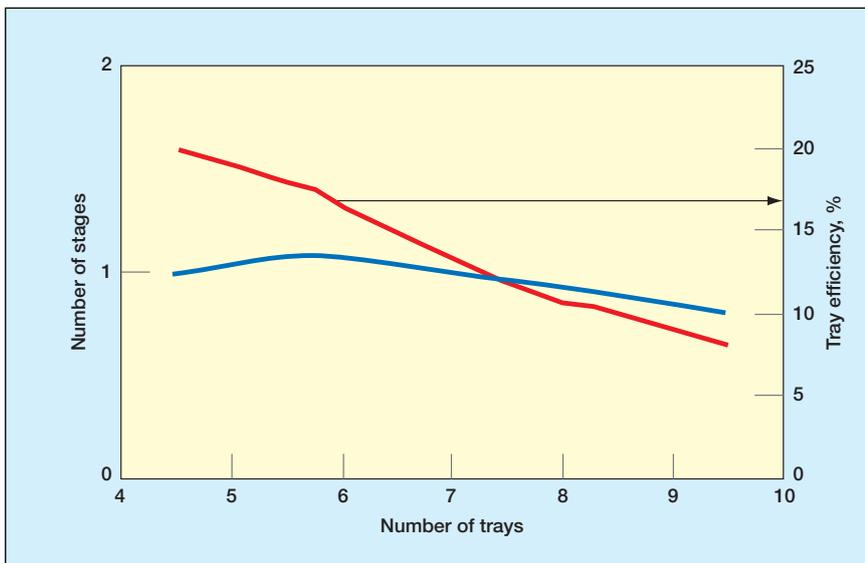
**Figure 7** An observed set of tray separation stages for different tray counts in operating vacuum units. The tray count appears to be insensitive to the actual number of stages (approximately one), represented in a reduced tray efficiency
