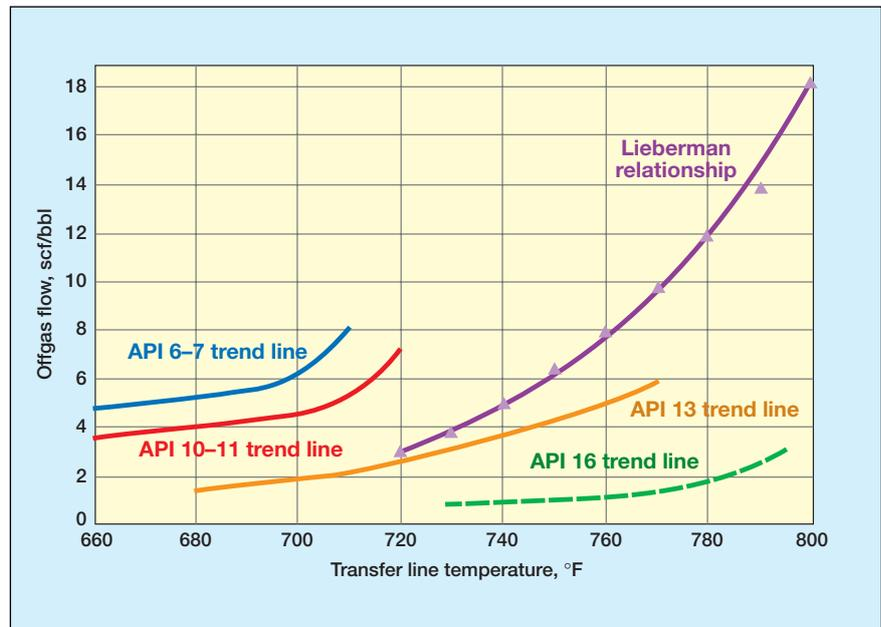
**Figure 4** Addition of heavier unconventional crude data sets to the transfer line to off-gas flow-to-crude flow ratio relationship. From the data illustrated, as the API decreases (heavier crude), the degree of cracked gas (translated to off-gas) increases
