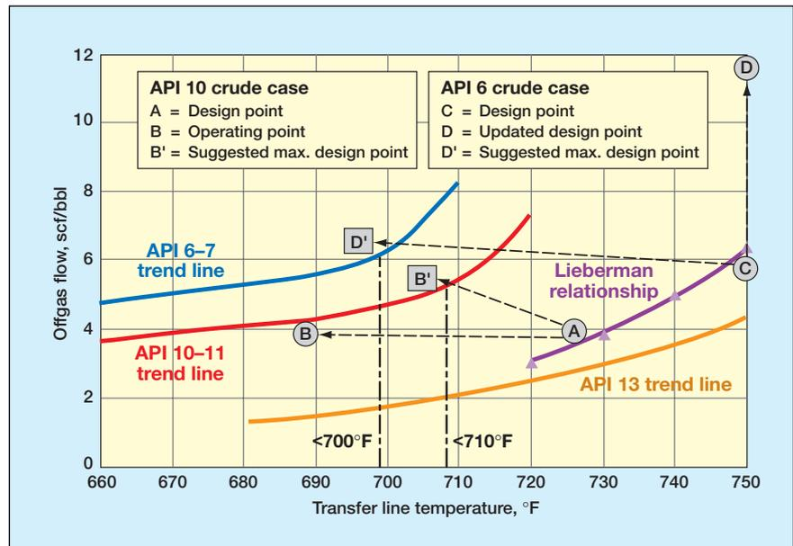
**Figure 5** Operating case: point A was a design point for an API 10 unconventional crude vacuum unit. The unit operated at point B, a lower heater outlet/transfer line temperature. Point B' is a possible design point. Design case: point C was a design point for an API 6 unconventional crude vacuum unit. The unit is now desired for point D, while point D' is suggested as a design point (reduced heater design temperature)
