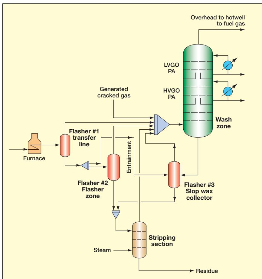
Figure 1 Proven vacuum column simulation topology to represent non-equilibrium tendency in feed to vacuum column.<sup>2</sup> Experience factors for bitumen-derived crude for cracked gas, entrainment and the stripping section should be provided to adequately represent actual operation
