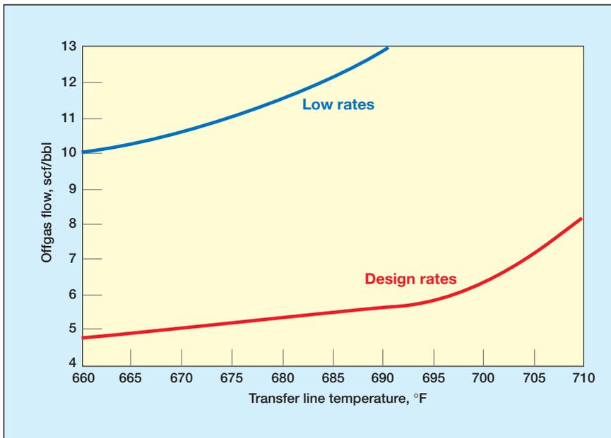
**Figure 6** Cracked gas make for an API 6–7 unconventional crude vacuum unit, comparing low feed rates (approximately 60–65% of design rates) to design feed rates. The off-gas flow per barrel of crude produced was nearly double for the low flow rates
