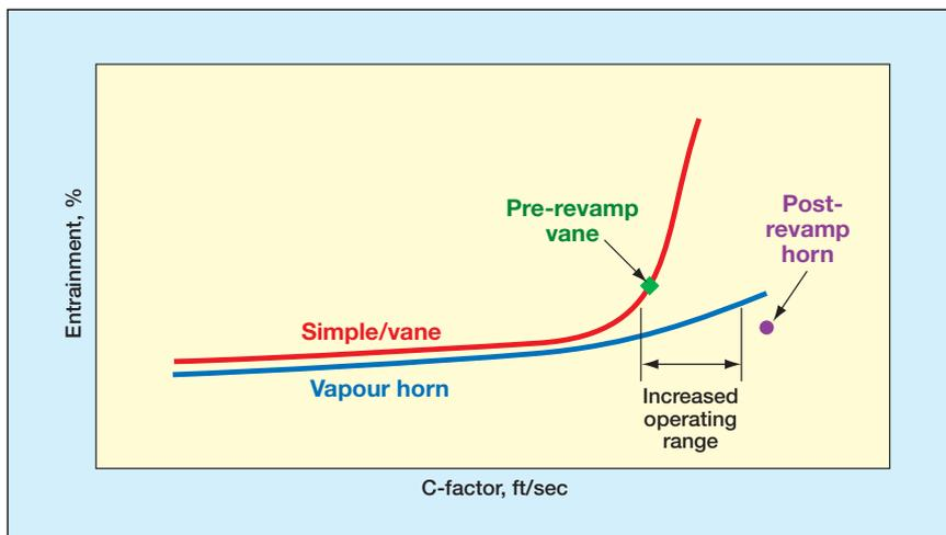
**Figure 8** CFD analysis validating actual operating points pre- and post-revamp of a vacuum tower feed inlet device. An enhanced vapour horn replaced an even flow inlet feed device, allowing an increase in unit feed rate while maintaining the HVGO product specification (by decreasing entrainment generated)
