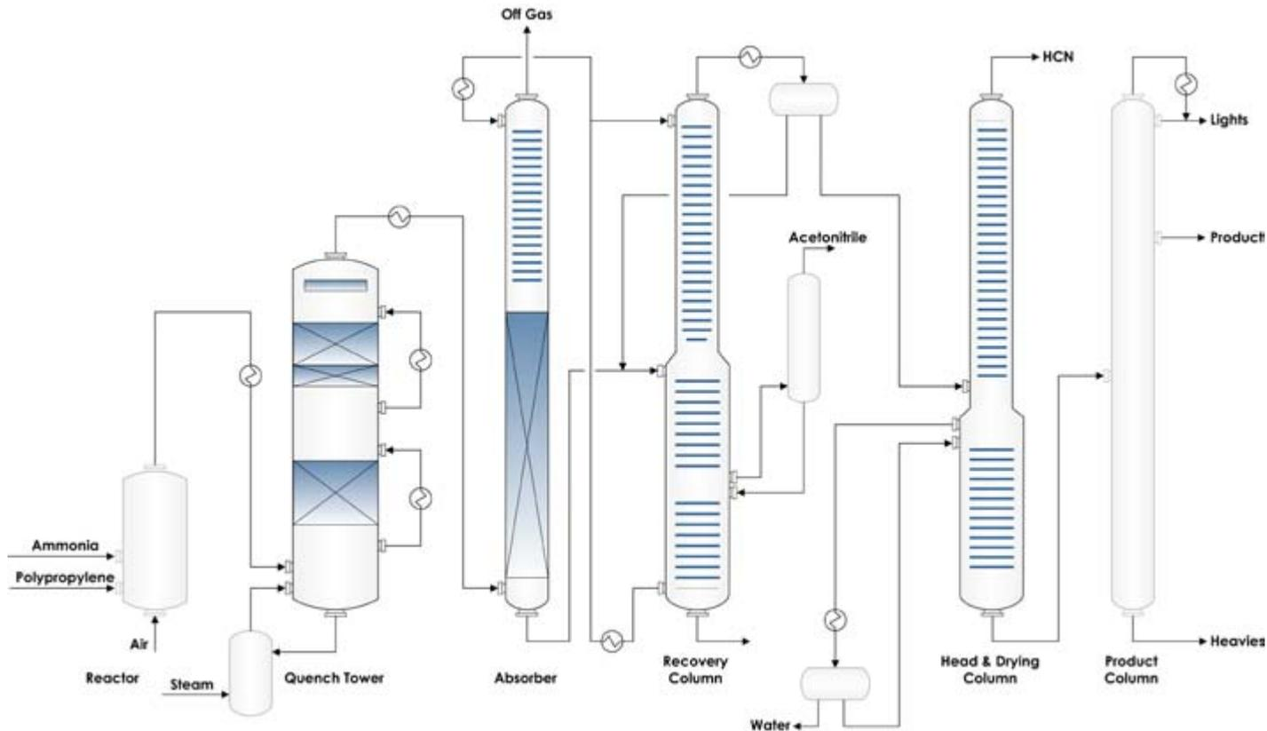
Polymerization and coking can cause major operational problems in an acrylonitrile plant, leading to premature shutdowns and lost production. Koch-Glitsch can provide a variety of internals to reduce or eliminate these problems.
