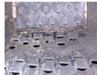
**PROVALVE® orifices show little signs of fouling after 5 months.**
