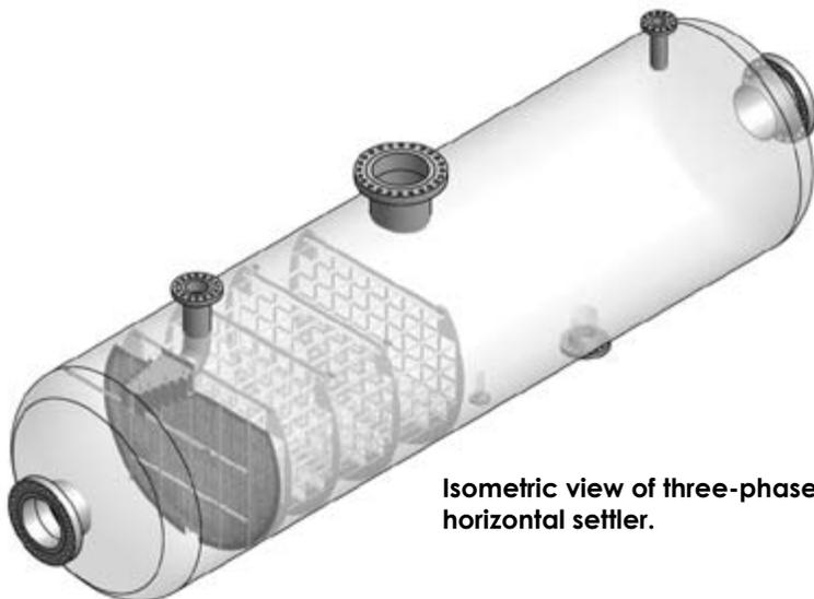
Isometric view of three-phase horizontal settler.
