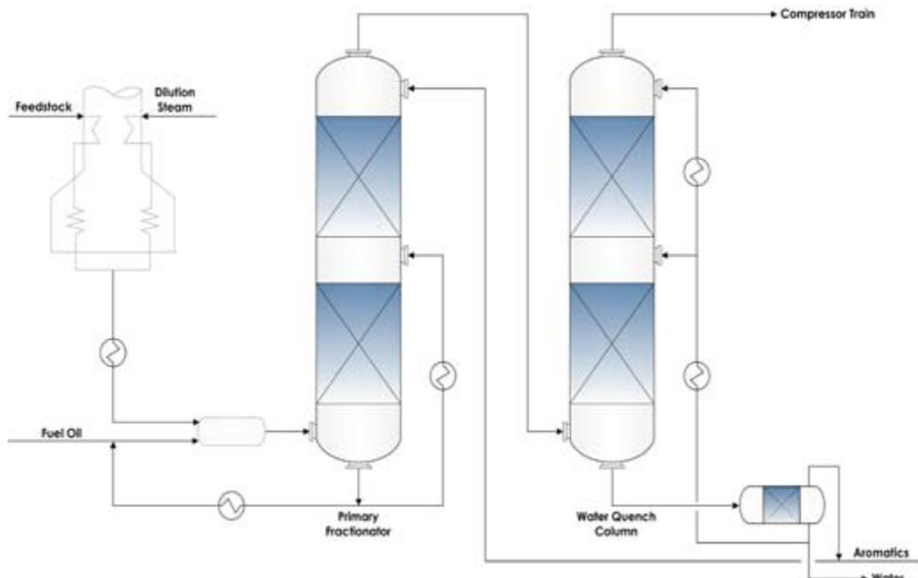
In Ethylene (Olefins) plants, significant fouling potential exists in the Quench columns that cool the hot process gas from the cracking furnaces. Coke fines from the cracker are entrained with the vapor to the first column in the Quench Unit. This first column will be an Oil Quench (Primary Fractionator) when cracking naphtha liquids or a Water Quench column for ethane or propane feedstocks.
