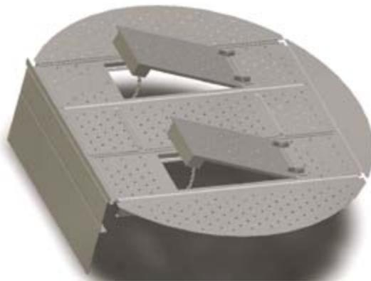
**Explosion doors can provide protection to trays during an upset.**
