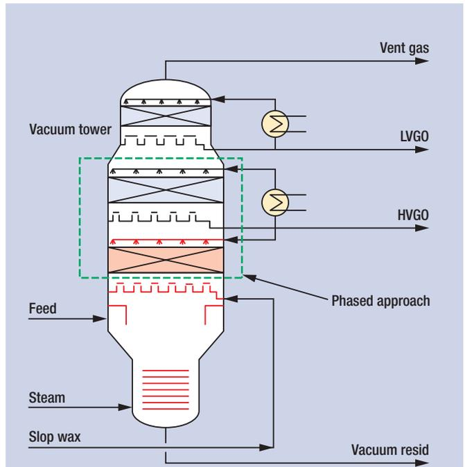
**FIG. 5** Vacuum column design using phased approach.
