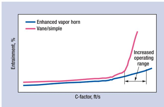
**FIG. 4** Inlet feed device relative performance comparison.
