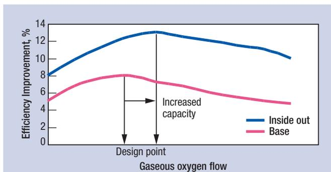
**FIG. 7** Performance differences between inside-out approach and standard design methodology.
