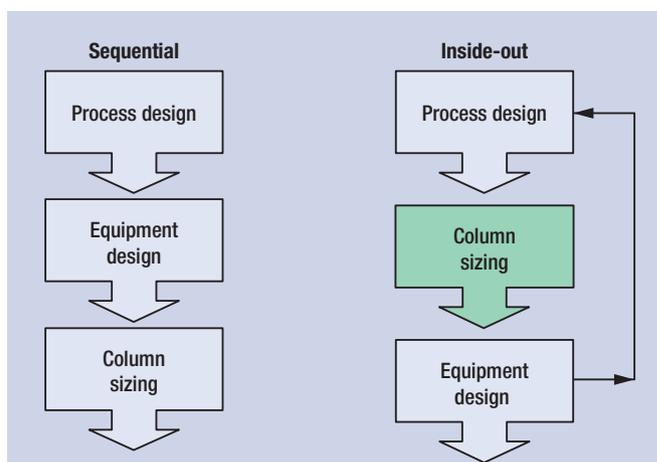
**FIG. 1** Sequential vs. inside-out approach for distillation unit design.
