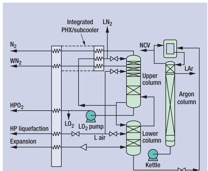
**FIG. 6** Schematic of a typical air separation unit.
