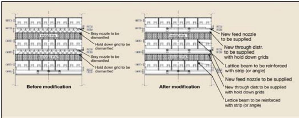
Figure 4 Details of the internals configuration pre- and post-revamp
