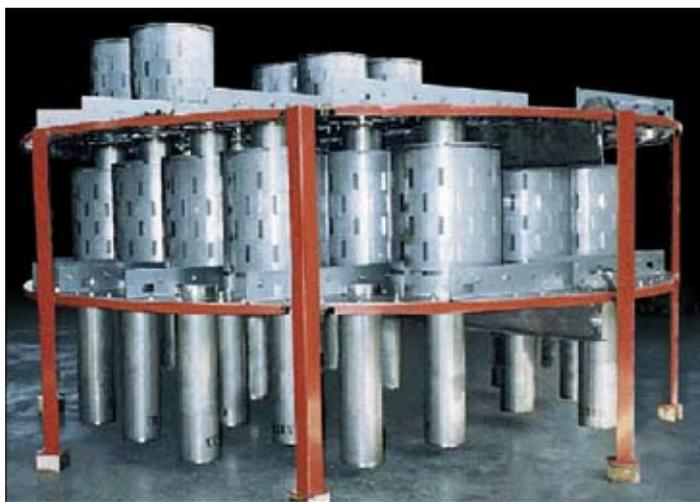
Figure 3 Setup of Ultra-Frac trays
