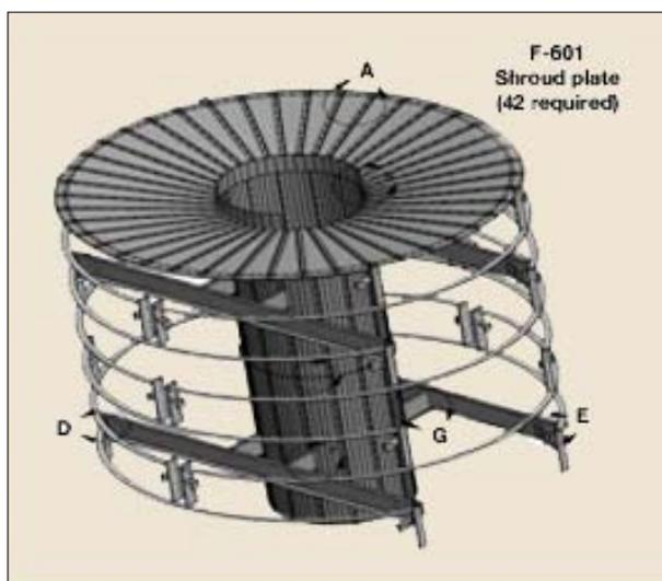
Figure 2 Modified stripping section — HDS fractionator
