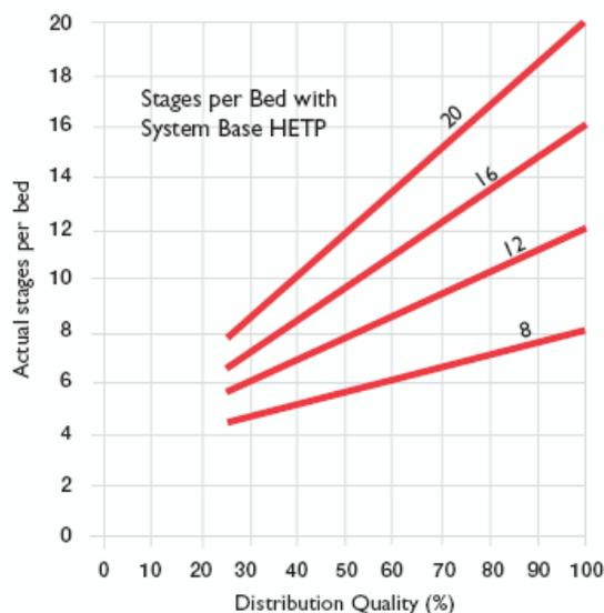
A tower containing deep beds of IMTP high efficiency random packing, designed to achieve many theoretical stages or transfer units, is very sensitive to liquid distribution quality.
