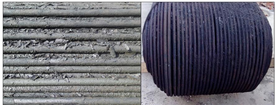
Figure 6 Fouled debutaniser reboiler tubes
