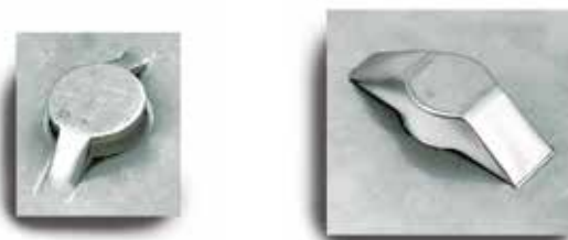
▲ Figure 6. The simplest fixed valve is an extruded hole and cover with small-diameter (left) or large-diameter (right) orifices.
