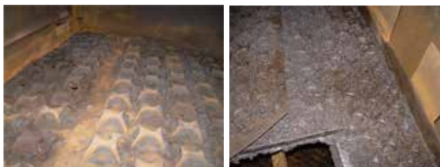
▲ Figure 15. After operating for one cycle in a coker fractionator, these moving caged valves had considerable fouling.
