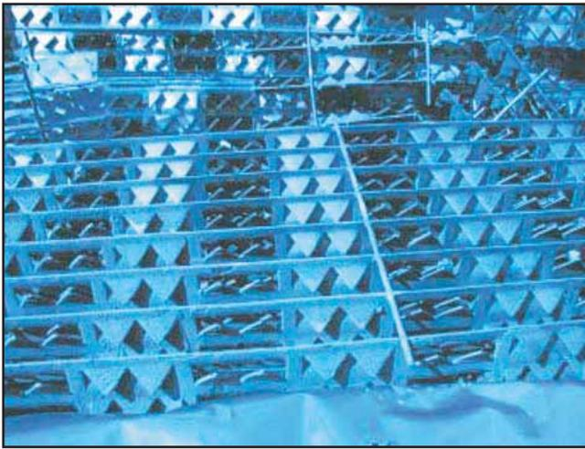
Figure 2 Flexigrid style 2 removed from slurry pumparound
