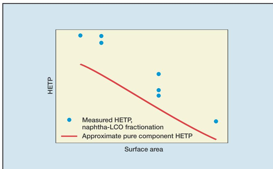
Figure 1 Measured HETP for structured packing in FCCU main fractionator naphtha-LCO fractionation
