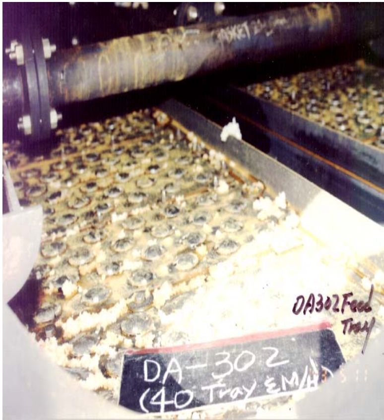
Fouled Valve Tray Before Revamp "Pop-corn Polymer"
