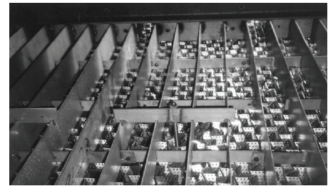
Hold down grid with through rod for a structured packing or grid bed.
