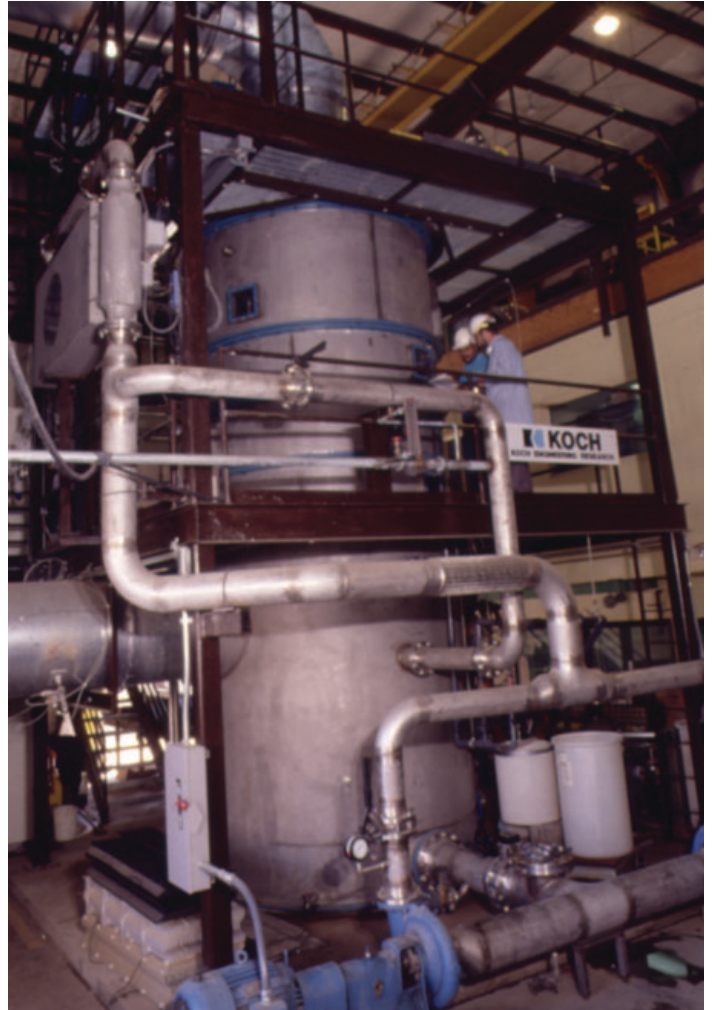
The 8ft. diameter test tower offers simulated performance in 1/8 scale.
