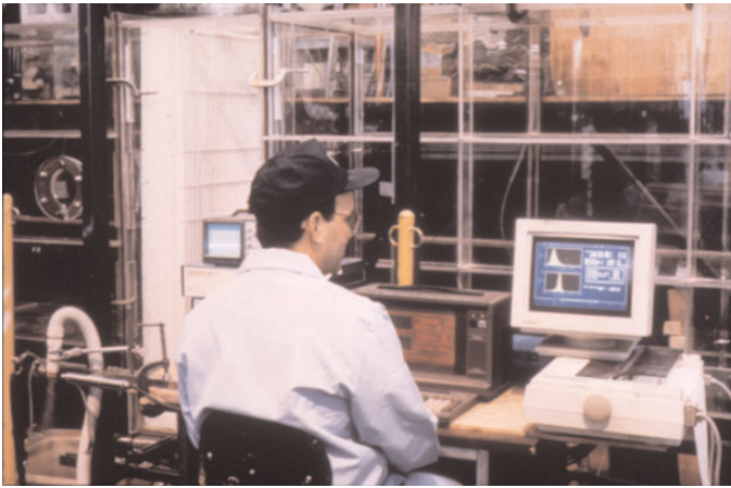
Using the Phase Doppler Particle Analyzer, performance data is taken in the horizontal flow test unit.
