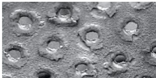
▲ Figure 13. Sieve trays in a solvent-recovery dehydration column experienced severe fouling after approximately 120 days in service.
