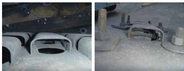
▲ Figure 16. Enhanced fixed valves had little fouling after being in service in a coker fractionator for several years.
