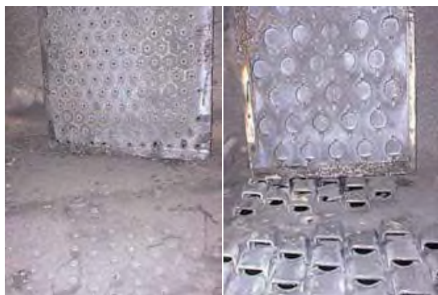
▲ Figure 11. After a sour-water stripper operated for a typical run length, the adjacent sieve (left) and enhanced-fixed-valve (right) trays were examined. The sieve trays had significantly more fouling than the fixed-valve trays.
