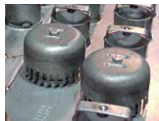
▲ Figure 2. A bubble-cap tray has risers on each hole with caps covering the risers.
